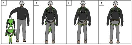
Once leg straps, waist belt (if applicable), and chest strap are buckled, use the adjusters to tighten or loosen harness until a snug fit is achieved:
