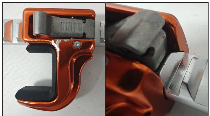
Deformed Release Lever:
