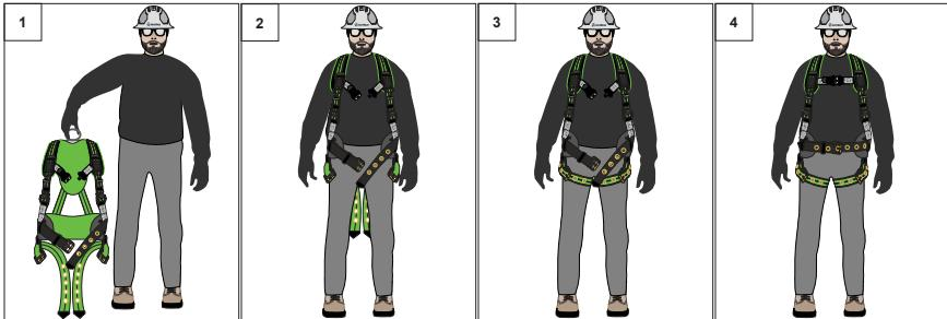
Once leg straps, waist belt (if applicable), and chest strap are buckled, use the adjusters to tighten or loosen harness until a snug fit is achieved. The harness should allow for a full range of movement. **Note:** Pass any excess strap webbing through plastic or elastic keepers.
