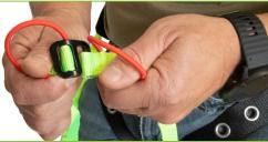
3B: Insert hook into soft loop slot at the end of the webbing fully. DO NOT HOOK ON THE RED ELASTIC RING.
