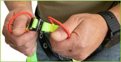
**3C**: Tug lightly on webbing to confirm hook is secure. Drop end without the hook ('B') and maintain hold of the webbing handle ('A') near the end with the hook.
