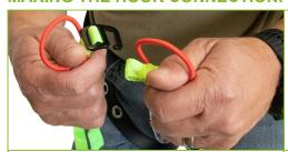
**3A**: Maintain a hold of red elastic rings. Raise the ends of the straps to identify hook and soft loop.
