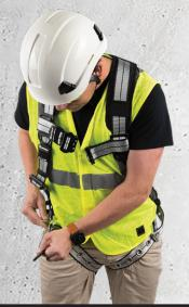
Pull leg straps between legs and connect to opposite ends. For a belted harness, connect waist strap after leg straps.
