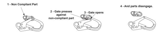
Using a connector that is undersized or irregular in shape (1) to connect a snap hook or carabiner could allow the connector to force open the gate of the snap hook or carabiner. When force is applied, the gate of the hook or carabiner presses against the non-compliant part (2) and forces open the gate (3). This allows the snap hook or carabiner to disengage (4) from the connection point.
