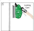
Place the Cable Sleeve onto the vertical cable so the cable is seated in the cable slot and release the locking lever and locking cam lever to complete attachment to the vertical cable (Figure 5).
