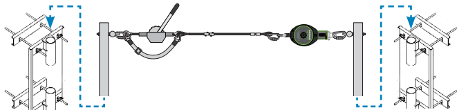
Fig. F. EZLink Double Connector (FS-EX2502-DBL) Attached directly to the column rebar cage—six (6) # 9 rebar or larger—without the need for decking alterations.
