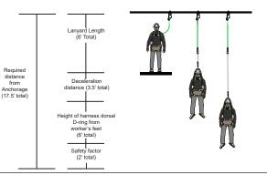
Swing Falls: Prior to installation or use, make considerations for eliminating or minimizing all swing fall hazards. Swing falls occur when the anchor is not directly above the location where a fall occurs. Always work as close to in line with the anchor point as possible. Swing falls significantly increase the likelihood of serious injury or death in the event of a fall. (See Figure 2)
