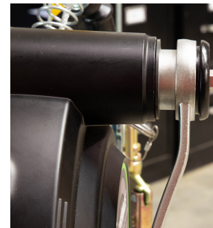
Crank Handle assembly pulled out in Self Retracting Device Configuration
