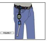
SW431 and SW432 elasticated lanyards are offered in 35 lbs capacity 50" to 62" length SW433 and SW434 elasticated lanyards are offered in 80 lbs capacity 66.5" to 80.5" length
