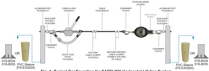
Fig. A. Typical Configuration for SAFELINK Horizontal Lifeline System PVC Sleeve is inserted into pre-poured concrete, and aluminum posts are inserted into PVC sleeve. (NOTE: Installation of the system with the FS-EX5501-5 Aluminum Posts is the only configuration that allows for (4) Users. All other installation methods that utilize other types of end anchorages are limited to (2) Users).
