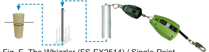
Fig. E. The Whizzler (FS-EX2514) / Single-Point Anchorage An aluminum cap with D-ring that swivels 360°. Used for single-point anchorage applications only (See pp. 8,9,12).
