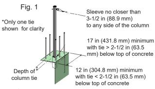
**RebarLink** The RebarLink Bracket is to be installed 6-1/2 ft (1.98 m) above the working surface. With the eye-bolt facing outward, place the bracket face perpendicular to the front of the rebar, centered on the cage. Slide the supplied cinching rebar bolts through both plates and tighten together with supplied wing nuts so that the Rebar Link is tightened onto the rebar cage
