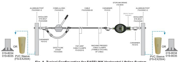
Fig. A. Typical Configuration for SAFELINK Horizontal Lifeline System PVC Sleeve is inserted into pre-poured concrete, and aluminum posts are inserted into PVC sleeve. (NOTE: Only this installation method allows for (4) Users. All other installation methods are limited to (2) Users).
