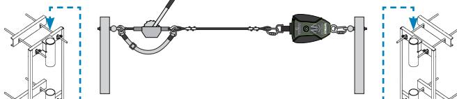
Fig. F. EZLink Double Connector (FS-EX2502-DBL)
