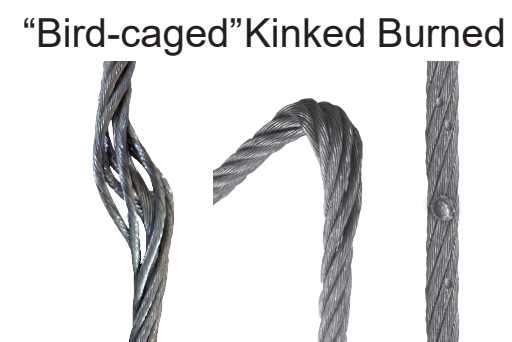
Fig. B: Cable Defects
