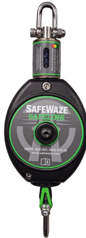
**Description** The SAFEWAZE™ StopLink Brake is an in-line energy absorber. It is designed to limit the maximum arrest load to no more than 1,000 lbf on end anchorages. Built-in tension indicator—Green = Spans up to 60 feet; Yellow = Spans over 60 feet; Red = Over-tensioned. Use only as outlined in the SafeLink User Manual. **If a fall occurs on the system, immediately remove from service and return to SAFEWAZE™ for authorized repairs or disposal.**
